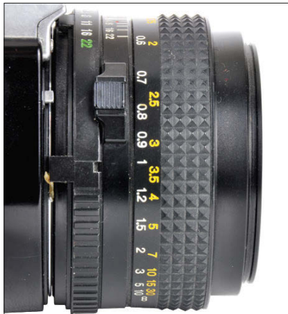
Focusing is normally carried out with a collar surrounding the lens barrel. (Minolta XD-7 camera)
